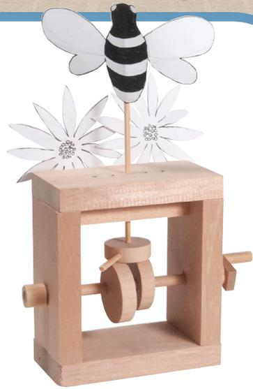
The handle turns the drive shaft which turns the round cams making the follower swing in a side to side movement while going up & down.
